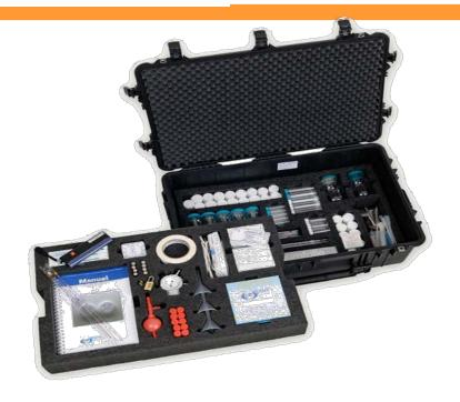
The Minilab<sup>®</sup> had been developed by GPHF in Germany as a simple, low tech and less expensive method for first quality screening of medicines. About 700 sets have been distributed to about 90 countries since 1997 by GPHF.
