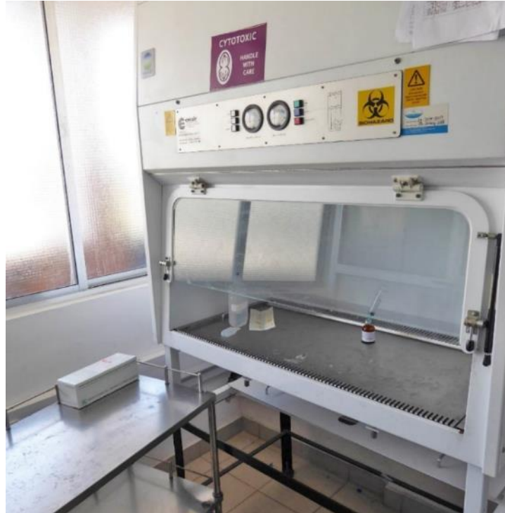
Figure 5: Cytotoxic safety cabinet (CSC) with HEPA filters and laminar air flow (© Peter Vollmer)
